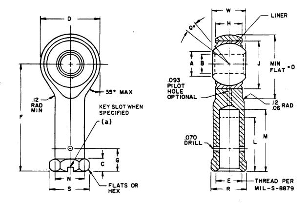
(a) For -3 thru -6, the keyslot shall be oriented perpendicular to the plane made by the face of the rod end hoop (see page 2 for additional details).
