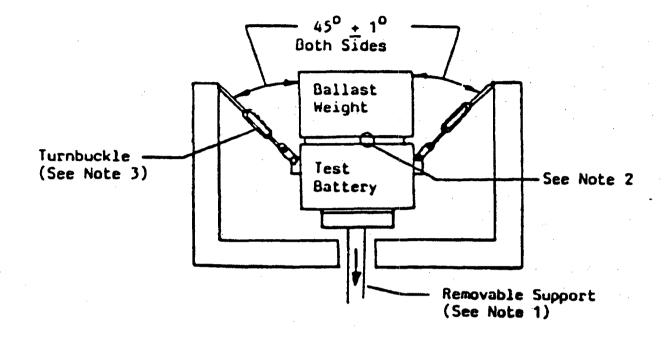
NOTES: 1. Support shallallow gradual and even removal so as to minimize shock and insure even loading of both handles.
