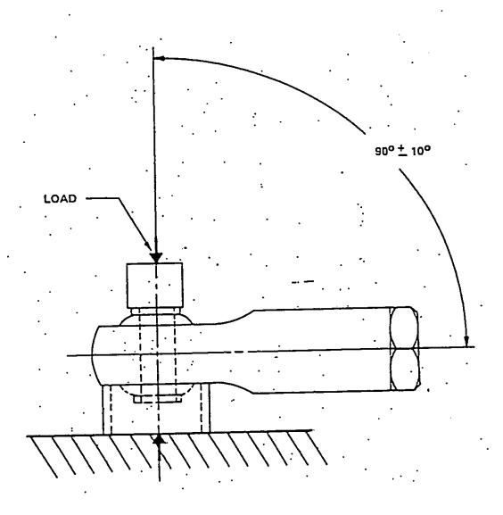
FIGURE 2. Axial Strength Test Setup
