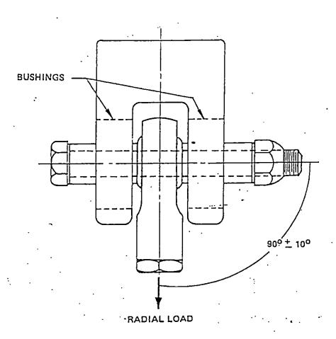
FIGURE 1. Radial Strength Test Setup
