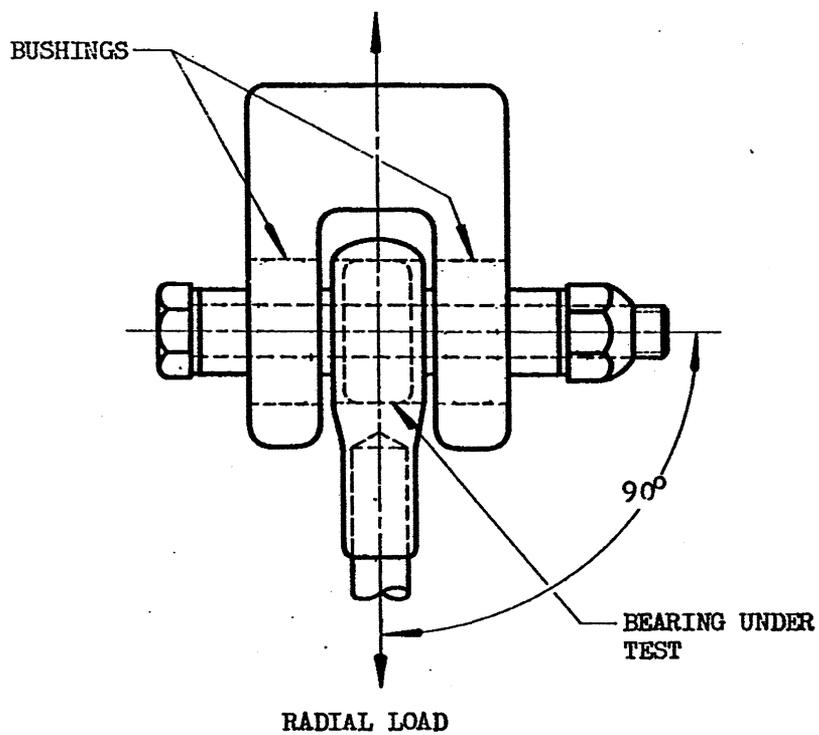
FIGURE 1. Radial Strength Test Set-up
