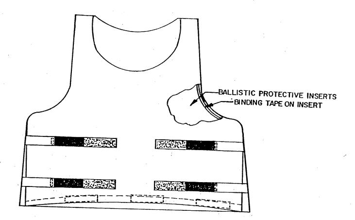
FIGURE 1: BODY ARMOR, FRAGMENTATION PROTECTIVE UNDERGARMENT, COMBAT VEHICLE CREWMEN'S
