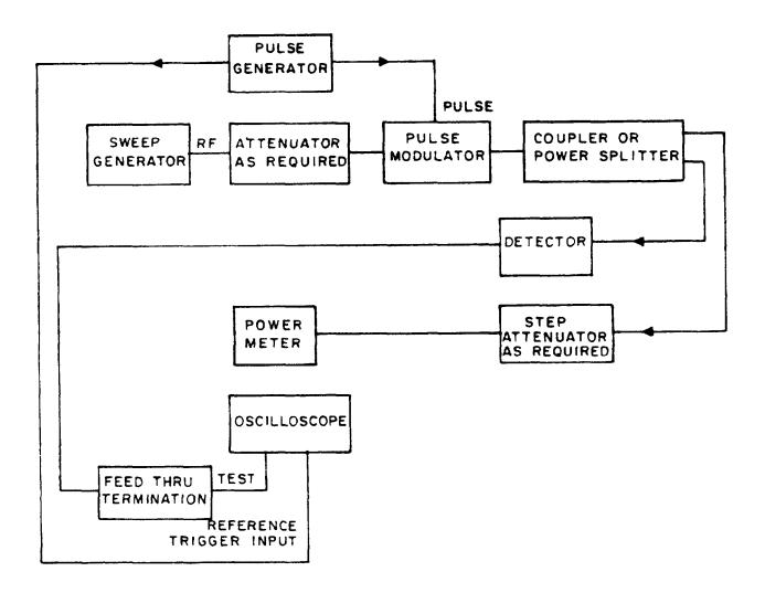
FIGURE 14A. Pulse response calibration setup.
