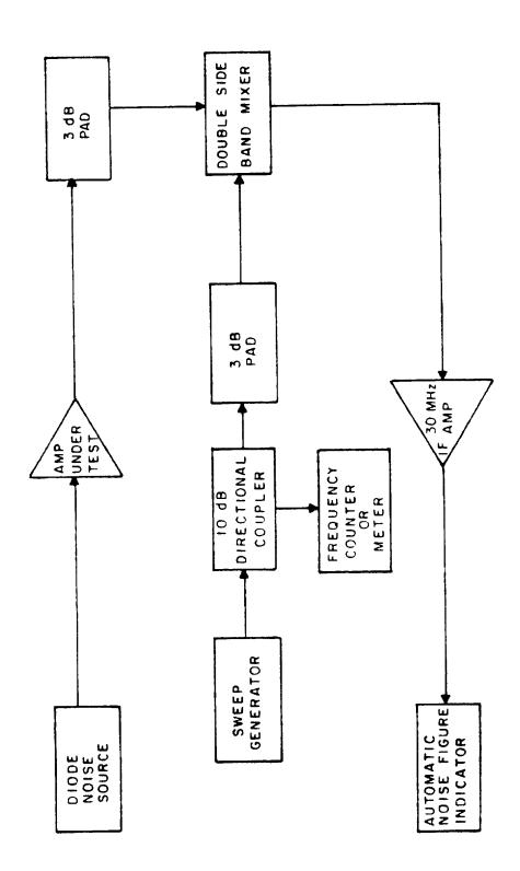
FIGURE 7. Noise figure > 3 dB test setup.
