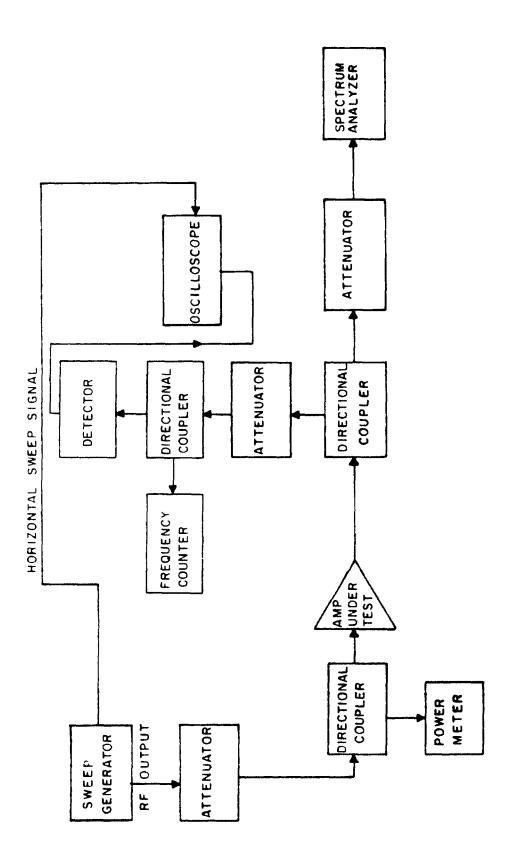
FIGURE 12. Harmonic and spurious test setup.
