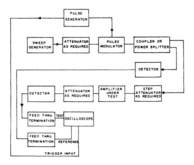
FIGURE 14B. Output pulse response test setup.
