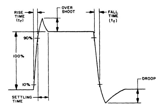
FIGURE 14. Pulse measurements.
