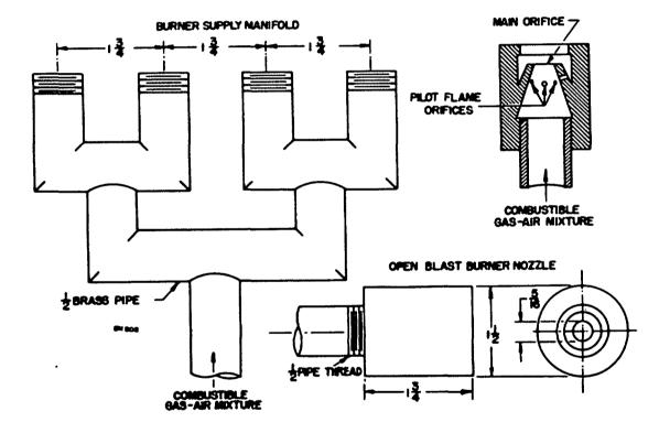
FIGURE 3. Burner supply manifold and open blast burner nozzle.
