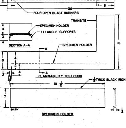
FIGURE 2. Detail of fire resistance test apparatus.
