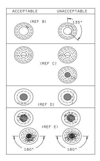
NOTE: The broken lines indicate the division of the radial distance between the terminal and the surrounding header metal into equal parts, thus creating concentric zones around the terminal.
