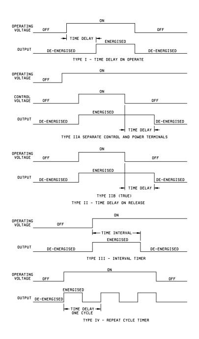
FIGURE 4. Relay timing diagrams.
