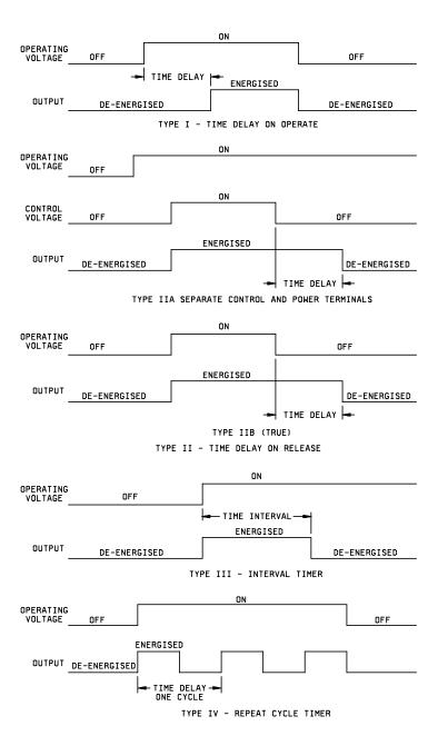
FIGURE 4. Relay timing diagrams.
