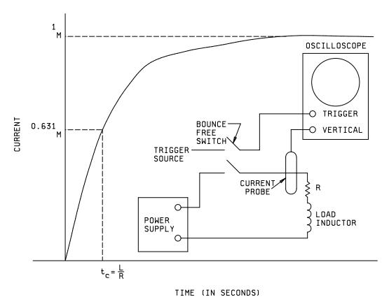
FIGURE 3. DC inductive load (inductive current rise time curve).
