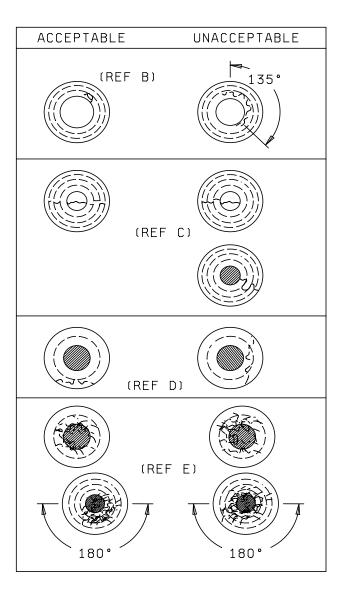
NOTE: The broken lines indicate the division of the radial distance between the terminal and the surrounding header metal into equal parts, thus creating concentric zones around the terminal.
