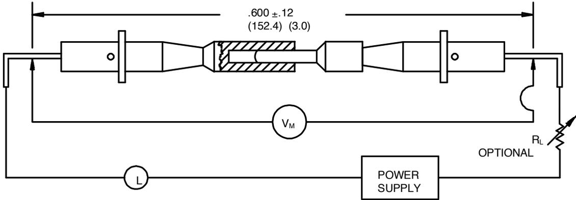
1. Voltage drop measurement connection points may be permanent connections and may be protected by potting or equivalents means.
