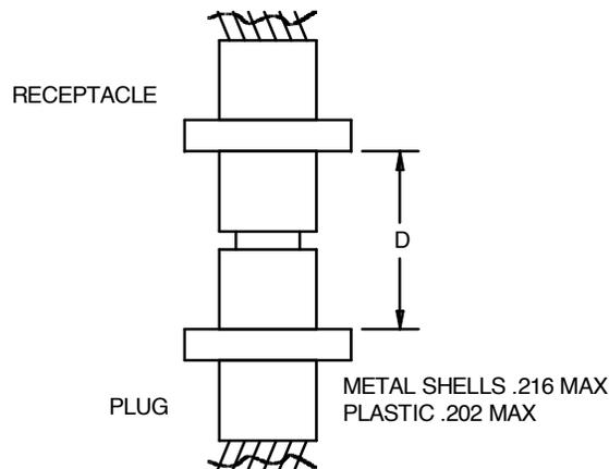
FIGURE 1. Connectors, fully mated.
