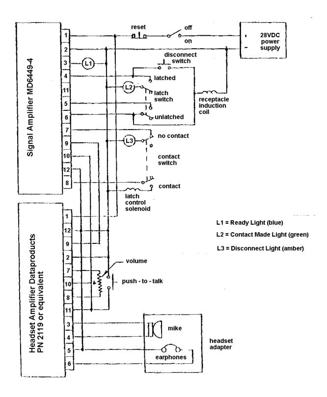
FIGURE 3. Functional Test Electrical Schematic
