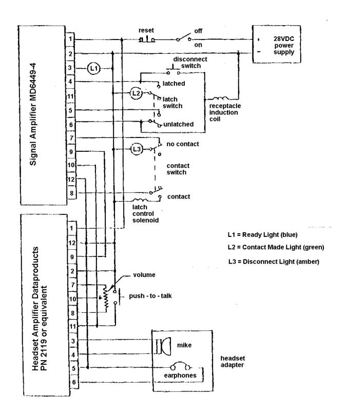
FIGURE 3. Functional Test Electrical Schematic
