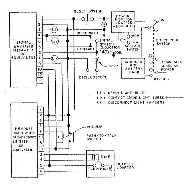
FIGURE 2. Tester Electrical Schematic
