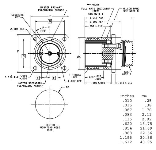
FIGURE 1. Wall mounting receptacle connector.
