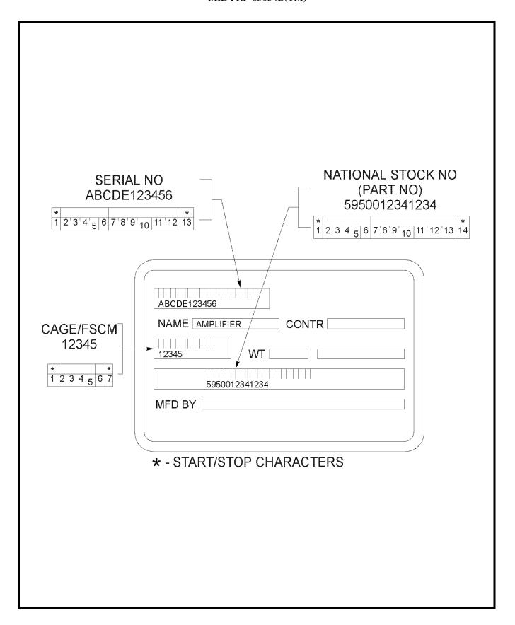
FIGURE 3. Example - ID plate with bar code.
