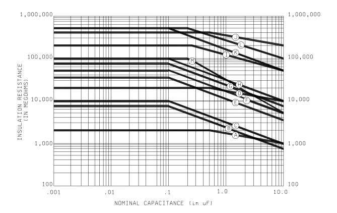
FIGURE 1. <u>Graphical representation of minimum insulation resistance</u>.
