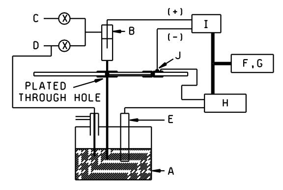
FIGURE E1. Schematic of SERA plated through hole apparatus.
