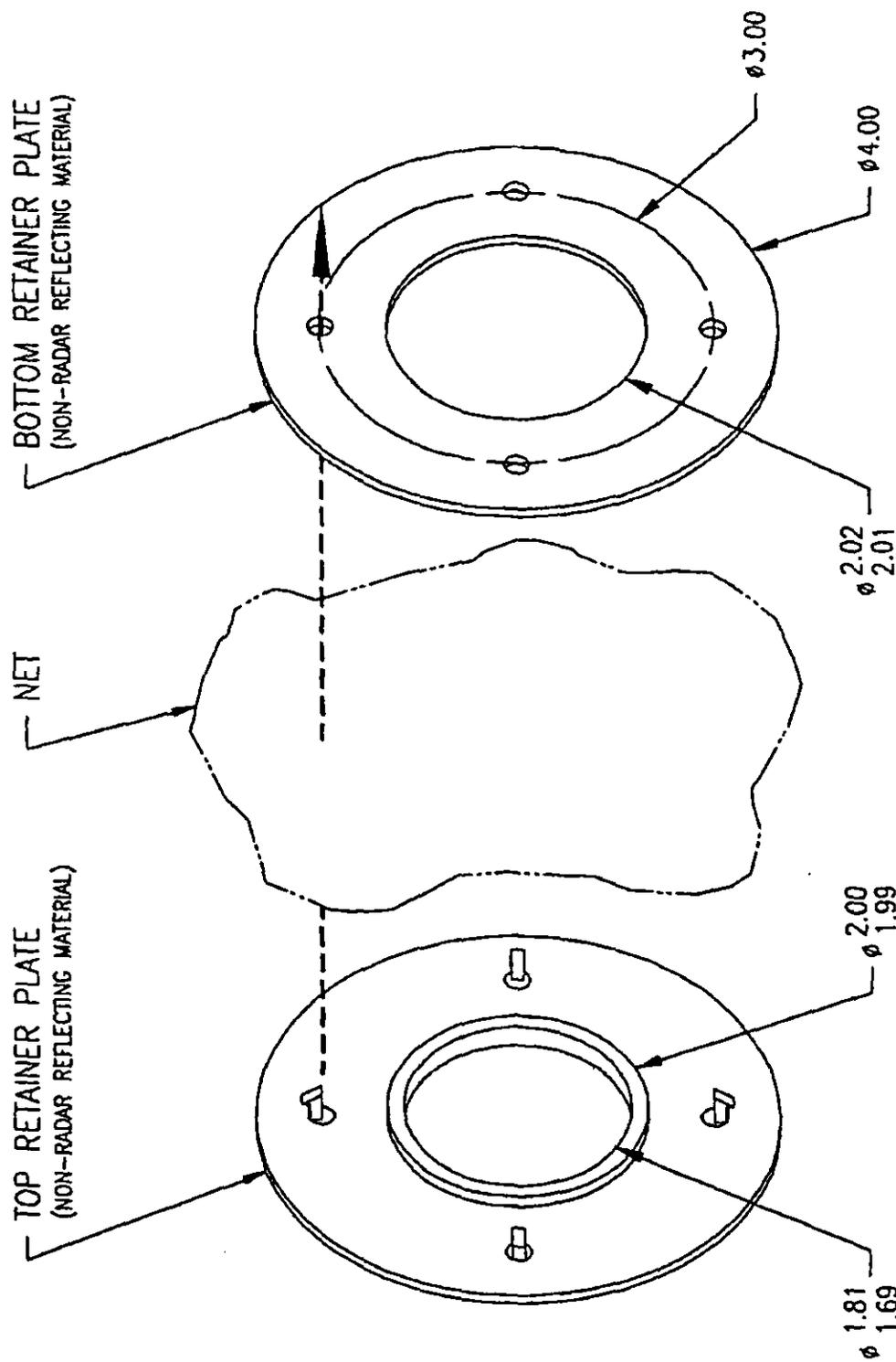
Figure 4. Antenna Flange Assembly
