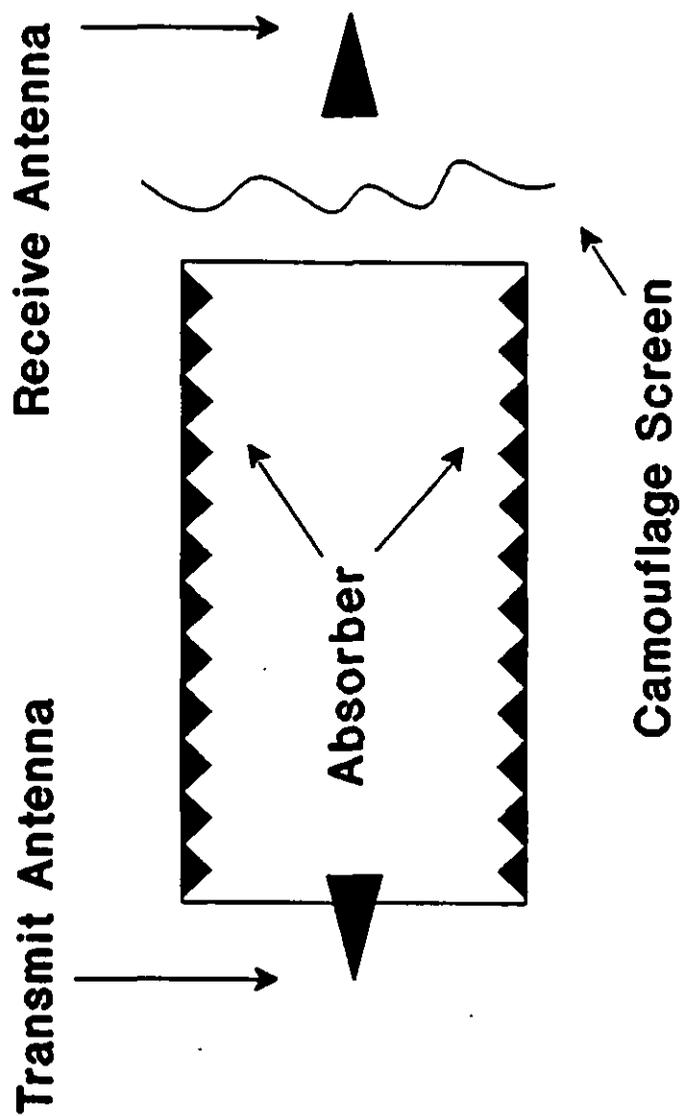
Figure 5. Admittance Tunnel
