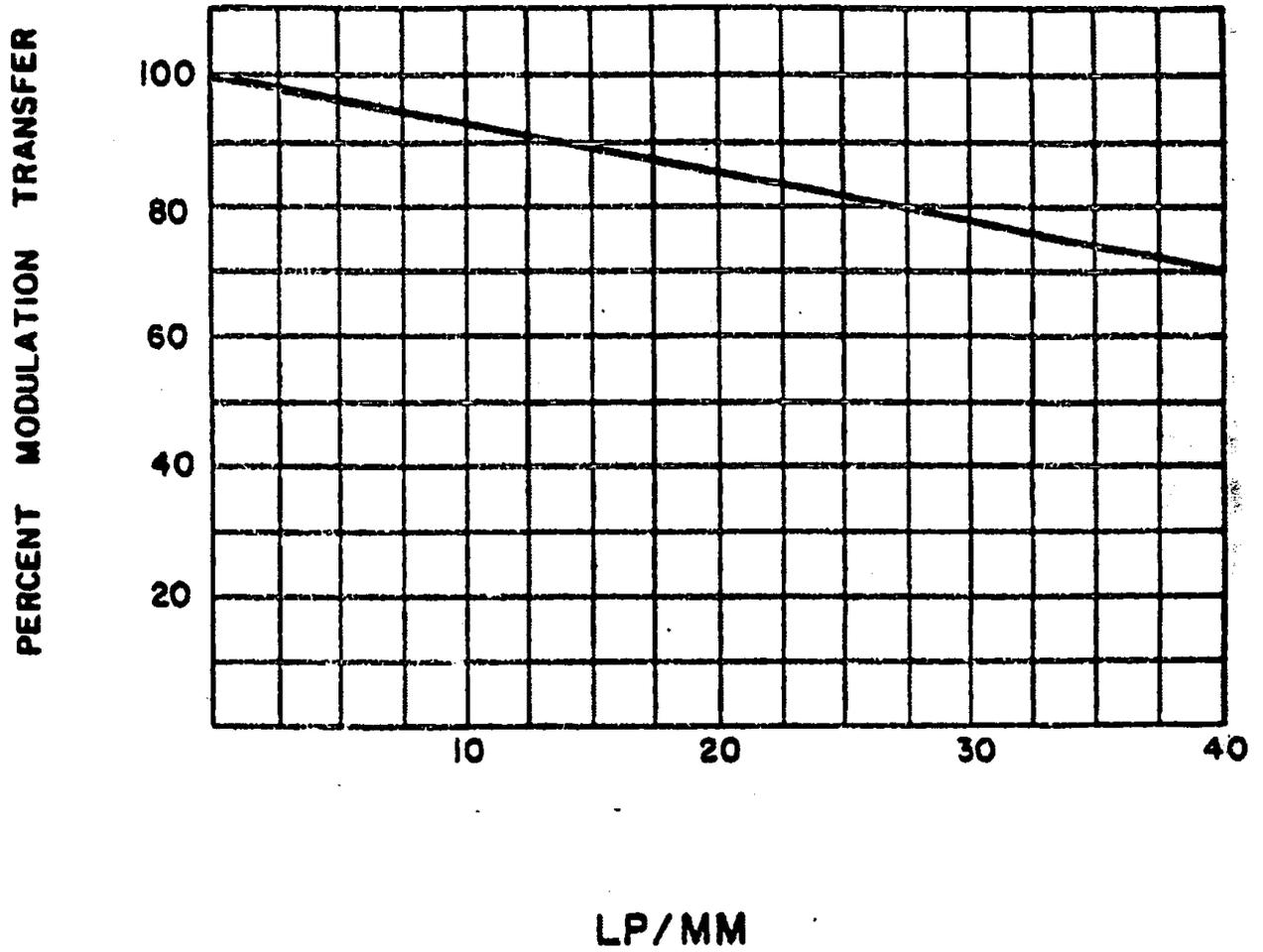
Figure 1. OBJECTIVE MTF ON AXIS
