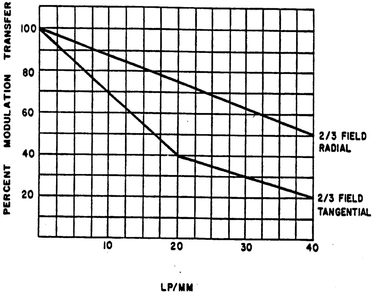
Figure 2. OBJECTIVE MTF OFF AXIS
