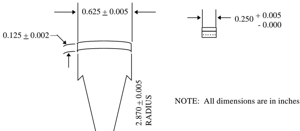
FIGURE 1. Shear test specimen.
