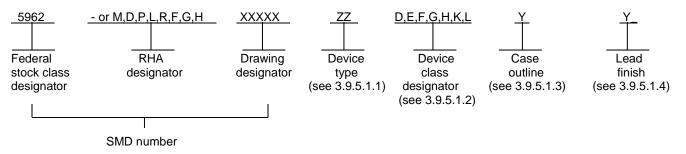
3.9.5.1.1 <u>Device type</u>. The device type shall identify the circuit function as indicated in the SMD.
