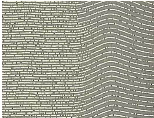
FIGURE 2. Undulating electrode and dielectric layers.
