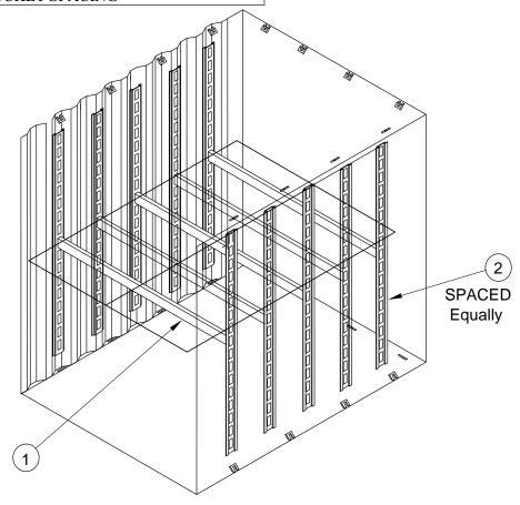
FIGURE 2. Tricon shelf decking support system.
