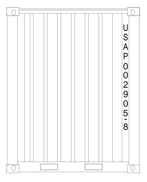
FIGURE 6. Aft wall of Type 1 Tricon; and door end without data plate for Type 2 Tricon marking example.
