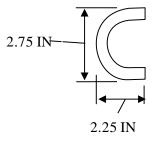
FIGURE 8. Loop tie down formed from 1/2-in (12.7 mm) steel rod.
