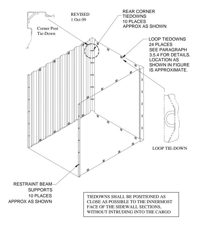
FIGURE 1. Tricon tiedown loop positions for Type I Tricon.
