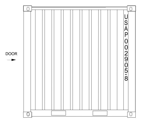
FIGURE 4. Right side view Tricon marking example.
