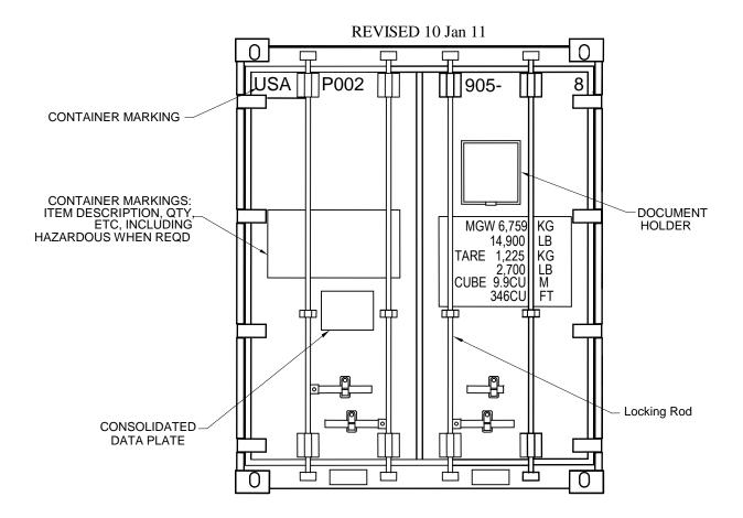
FIGURE 3. Tricon markings example.
