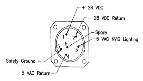
FIGURE 2. Wiring.
