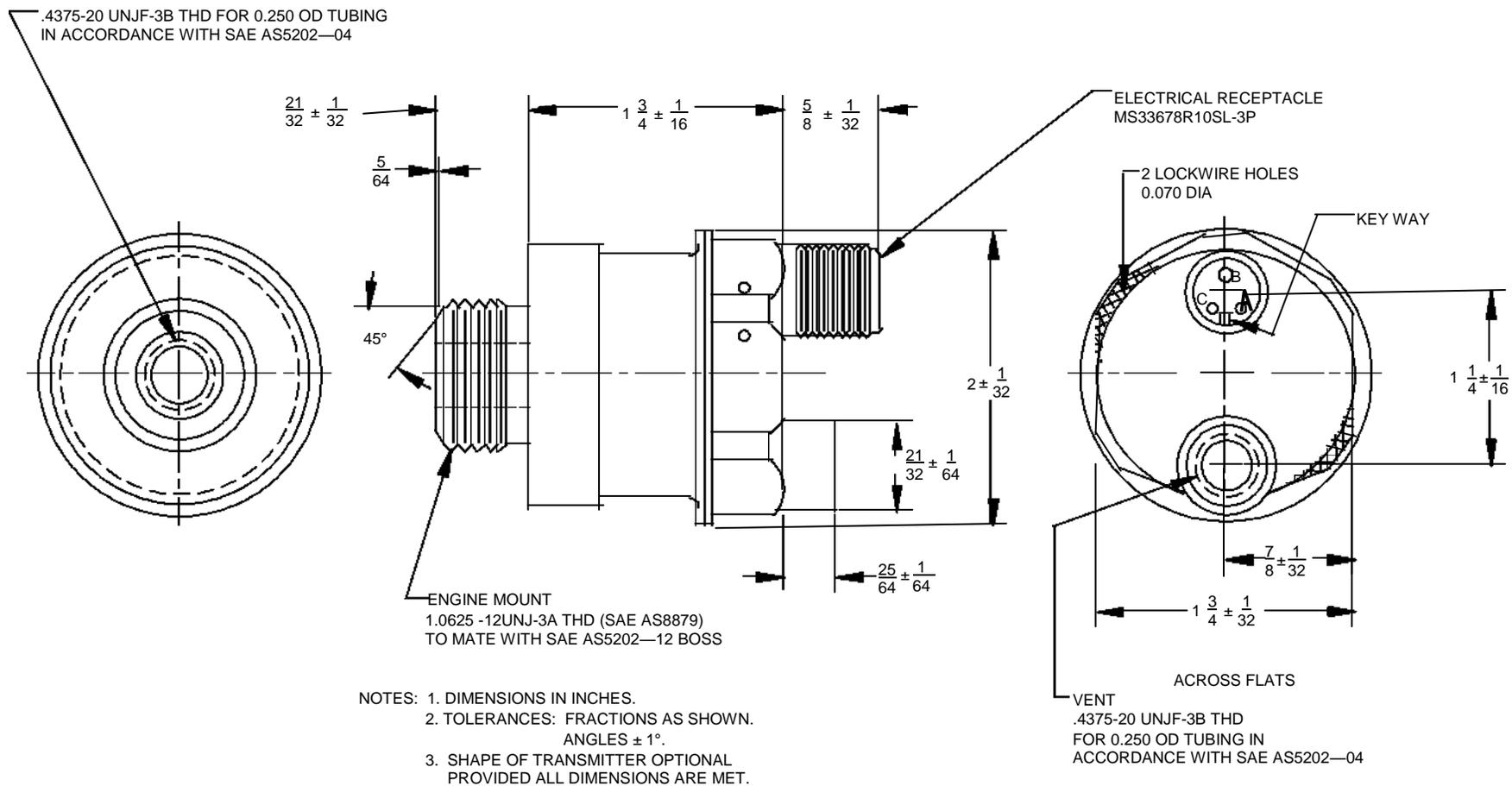
Figure 1. Transmitter case
