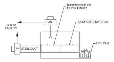
The purpose of the test is to assess the structural integrity and the smoke characteristics of the composite material separating the ship's internal compartments from the air flow within the confines of the composite envelope. Gases released to weather are also assessed as they can be reingested into the ship.
