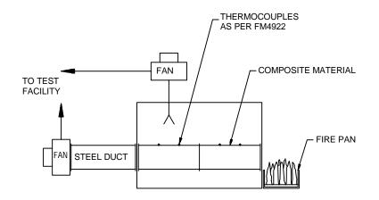
The purpose of the test is to assess the structural integrity and the smoke characteristics of the composite material separating the ship's internal compartments from the air flow within the confines of the composite envelope. Gases released to weather are also assessed as they can be reingested into the ship.
