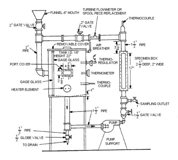
FIGURE 1. Corrosion test apparatus.
