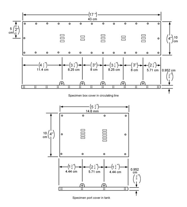
FIGURE 2. Specimen covers in corrosion test apparatus.
