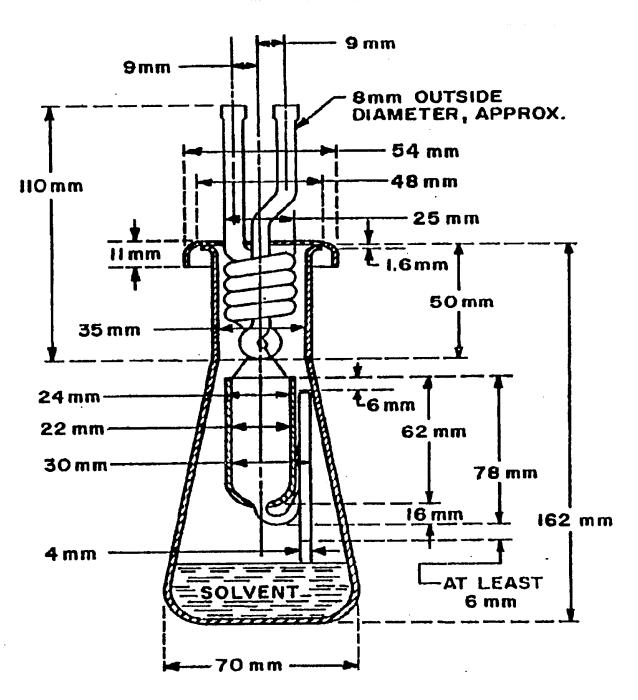
FIGURE 1. Extraction equipment.
