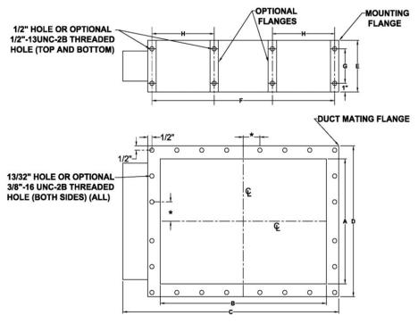
\* NOTE: IF THIS DIMENSION EXCEEDS 2 INCHES, PROVIDE HOLE ON CENTER LINE
