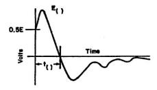
NOTE: The test sample shall be subjected to the spike(s) with the waveform shown and with the specified valtage (s) and pulsewidth (s).
