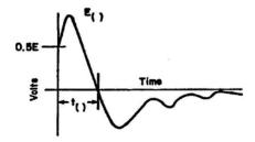
NOTE: The test sample shall be subjected to the spike(s) with the waveform shown and with the specified voltage(s) and pulsewidth(s).
