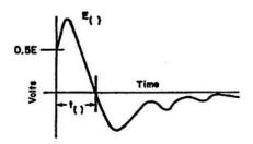
NOTE: The test sample shall be subjected to the spike(s) with the waveform shown and with the specified voltage (s) and pulsewidth (s).
