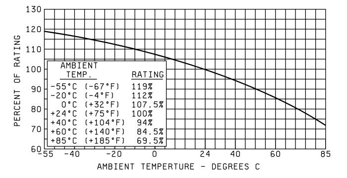
FIGURE 2. (FOR REFERENCE ONLY) - Effect of ambient temperature on the current carrying capacity of time-delay fuses (characteristic B).
