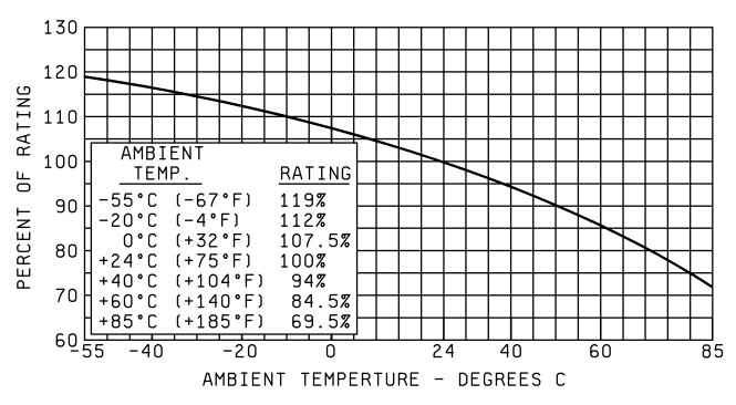
FIGURE 2. (FOR REFERENCE ONLY) - Effect of ambient temperature on the current carrying capacity of time-delay fuses (characteristic B).
