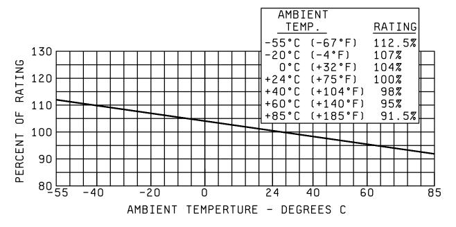
FIGURE 1. (FOR REFERENCE ONLY) - <u>Effect of ambient temperature on the current carrying capacity of normal fuses</u> (characteristic A and characteristic C).
