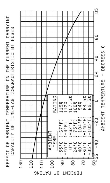
FIGURE 2. Effect of ambient temperature on the current carrying capacity of time-lag fuses (characteristic B).
