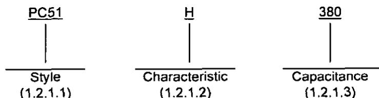
1.2.1.1 Style. The style is identified by the two-letter symbol "PC" followed by a two-digit number; the letters identify tubular-trimmer, piston-type, variable capacitors, and the number identifies the shape or differentiating electrical characteristics of the capacitor.
