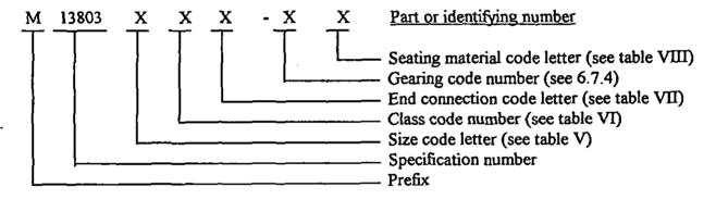
Example: M13803-D2A1B is the definitive specification part number for 8-inch (D), 150-class (2), cast-iron or steel double-disk gate valves (M13803) with flanged ends (A), spur gearing (1), and 18-8 chromium-nickel alloy steel seating material (B).
