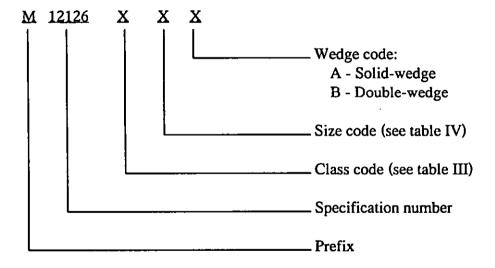
Example: M12126A2B is the part number for a lever operated bronze gate valve, (A) class 1 (125 psi), (2) size 1.5-inch, (B) double wedge conforming to MIL-PRF-12126.
