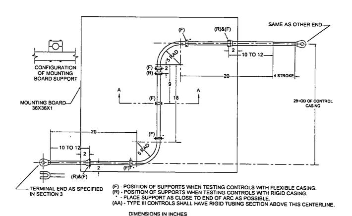
FIGURE 1. Push-pull control performance setup
