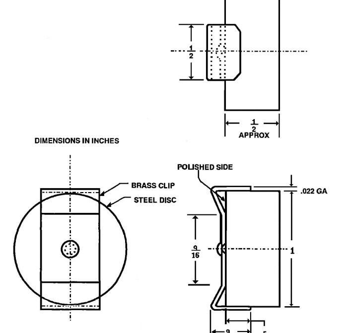
Figure 1. Typical test specimens for corrosivity test
