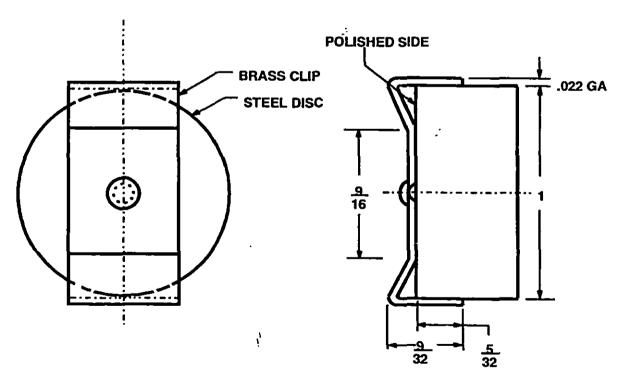
FIGURE 1. Typical test specimens for corrosivity test.
