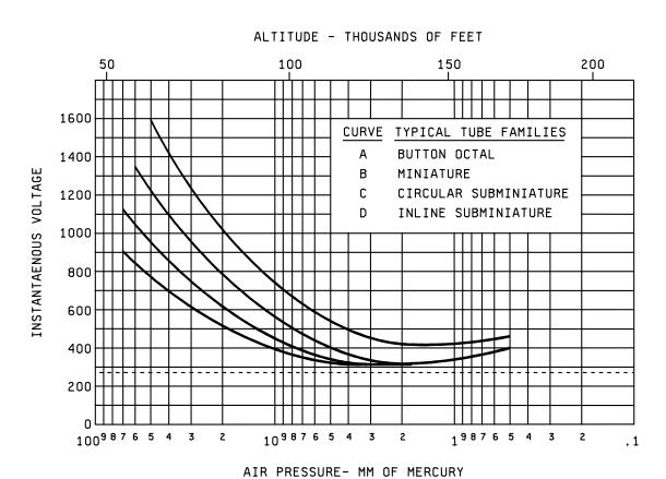
FIGURE 1. Reduced pressure (altitude) voltage breakdown characteristics.
