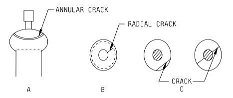
(2) Shaled seals or seals with cracks which fall outside the above limits.....
