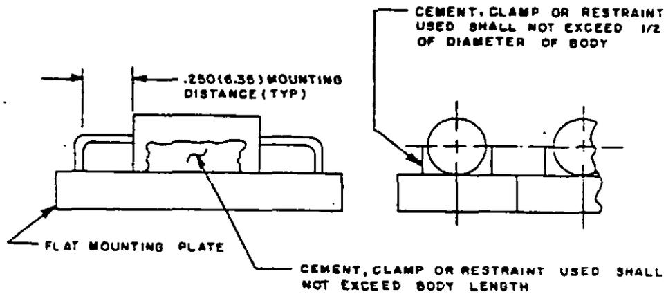
Mounting means for axial leaded resistors.
