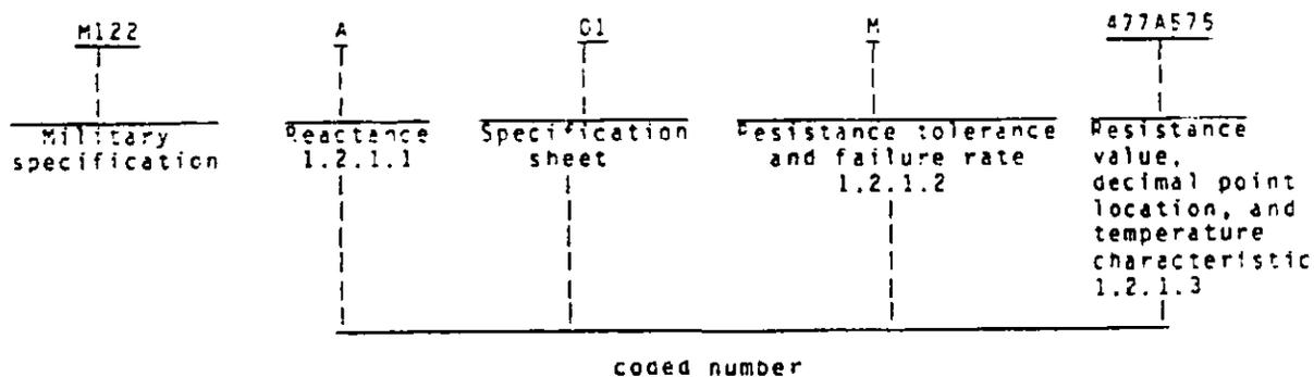
1.2.1.1 Reactance. The reactance is identified by a single letter in accordance with Table 1.
