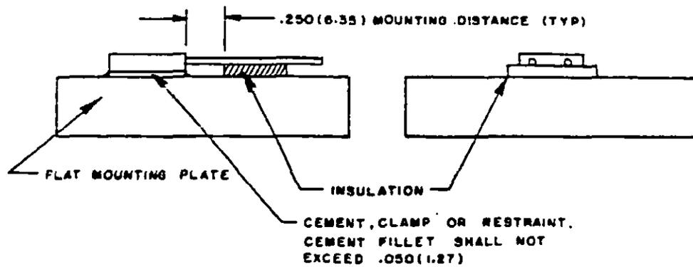
Mounting means for radial leaded resistors.
