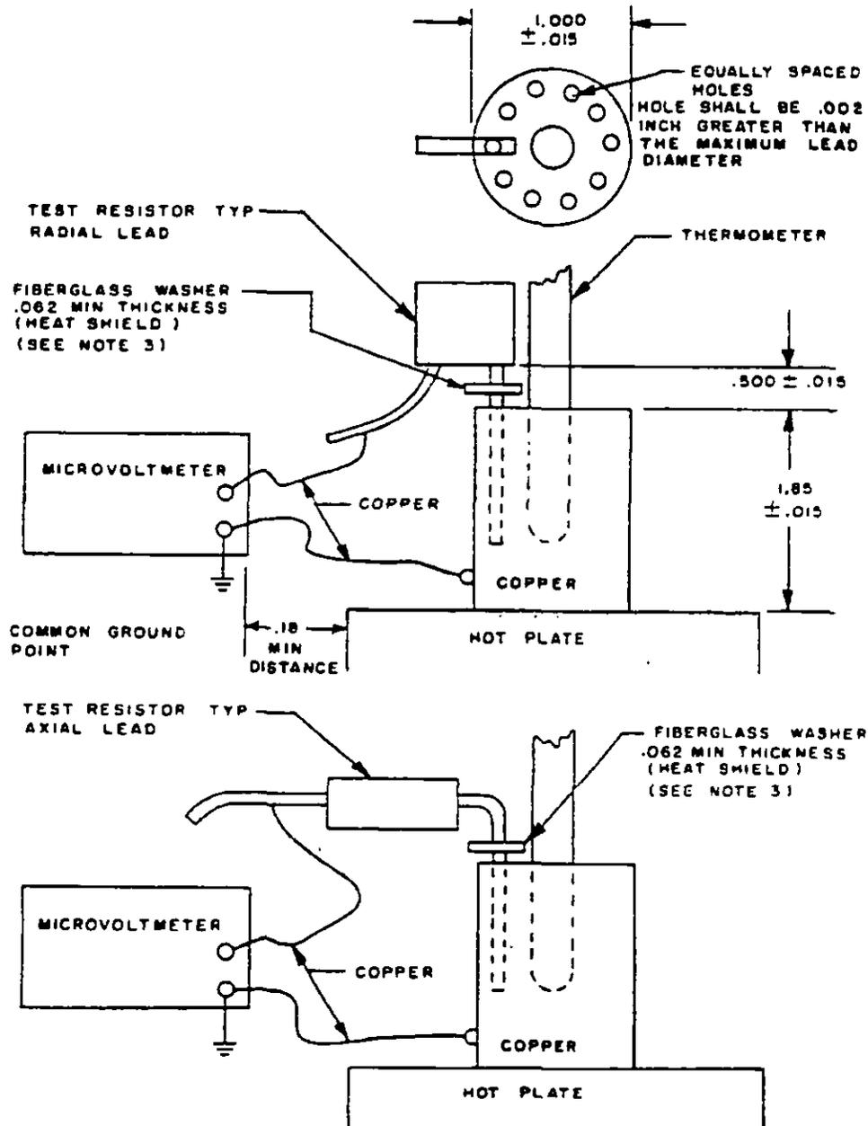
FIGURE 5. Thermal EMF test apparatus.
