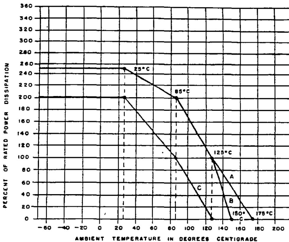
NOTE: These curves indicate the percentage of nominal wattage to be applied at temperatures higher and lower than 125°C for the same  $\Delta R$  change that would occur at 125°C during life testing (see 3.24). However, at no time shall the applied voltage exceed the maximum for each style (see 3.1).
