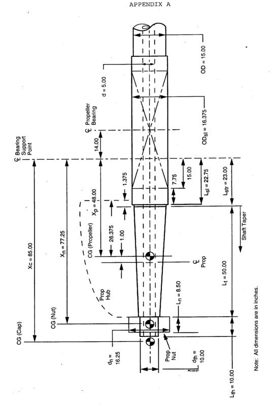
Figure 7. Submarine Shafting System: Aftermost Bearing Support Point
