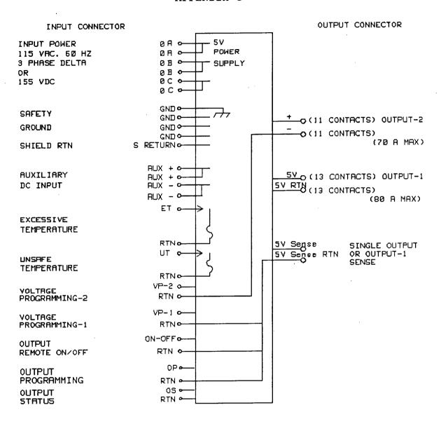
FIGURE 6. Example of an SPSP function diagram.
