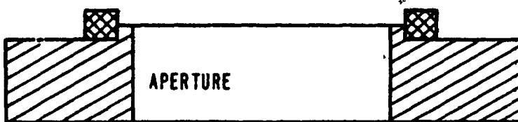
C. POSITIONED BY SHOULDER
