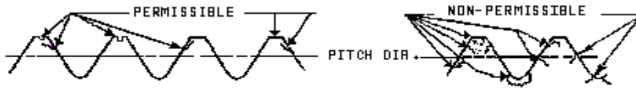
FIGURE 108-2. Laps and surface discontinuities.
