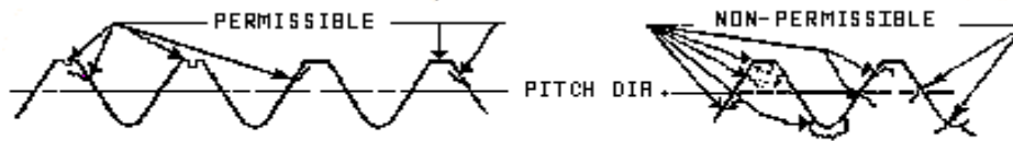
FIGURE 108-2. Laps and surface discontinuities.
