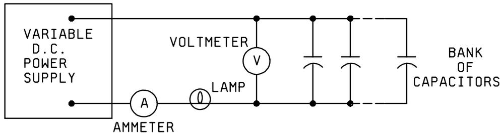
FIGURE 1. Schematic diagram.
