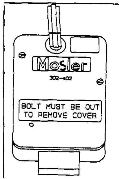
Figure 35 Mosler MRK 302-402 Backplate with Change Key in Inserted Position
