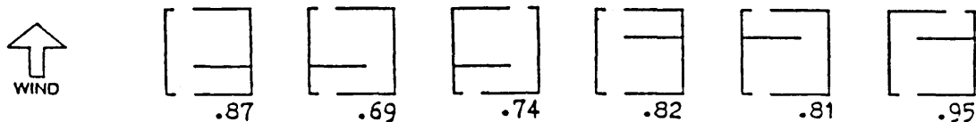
Figure C-5 Interior Partition Resistance Factors
