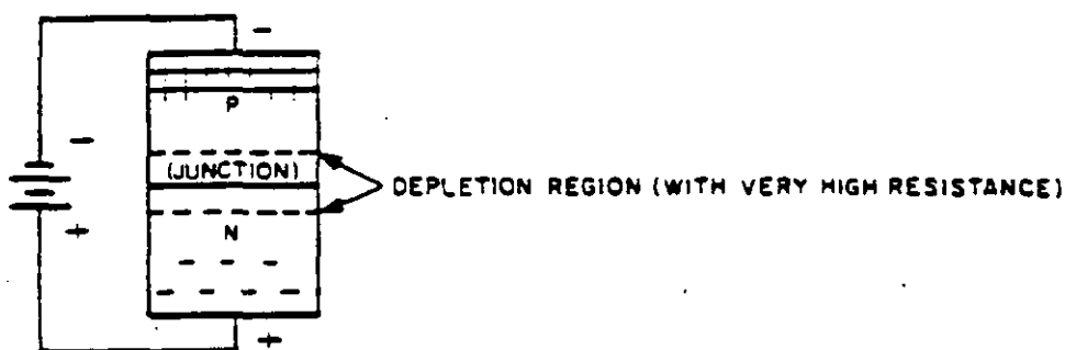
FIGURE 79. Basic silicon pn junction.
