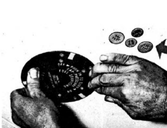
1. Remove pressure refueling cap.
